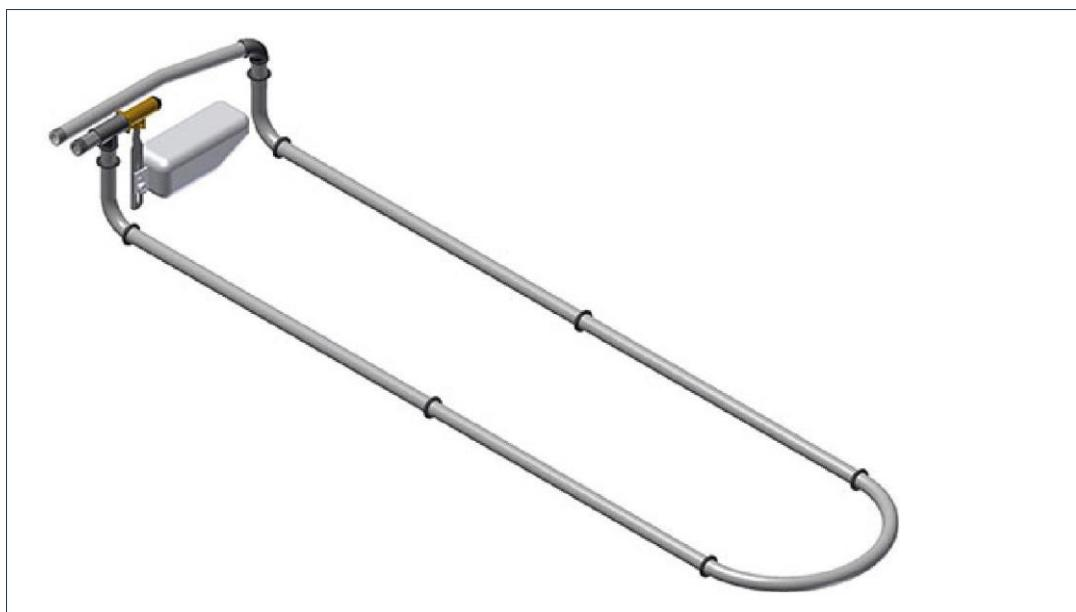
The optional circulation pipe prevents the water in the drinking trough from freezing by circulating water through the drinking trough. The supply pipe is mounted before the float.
